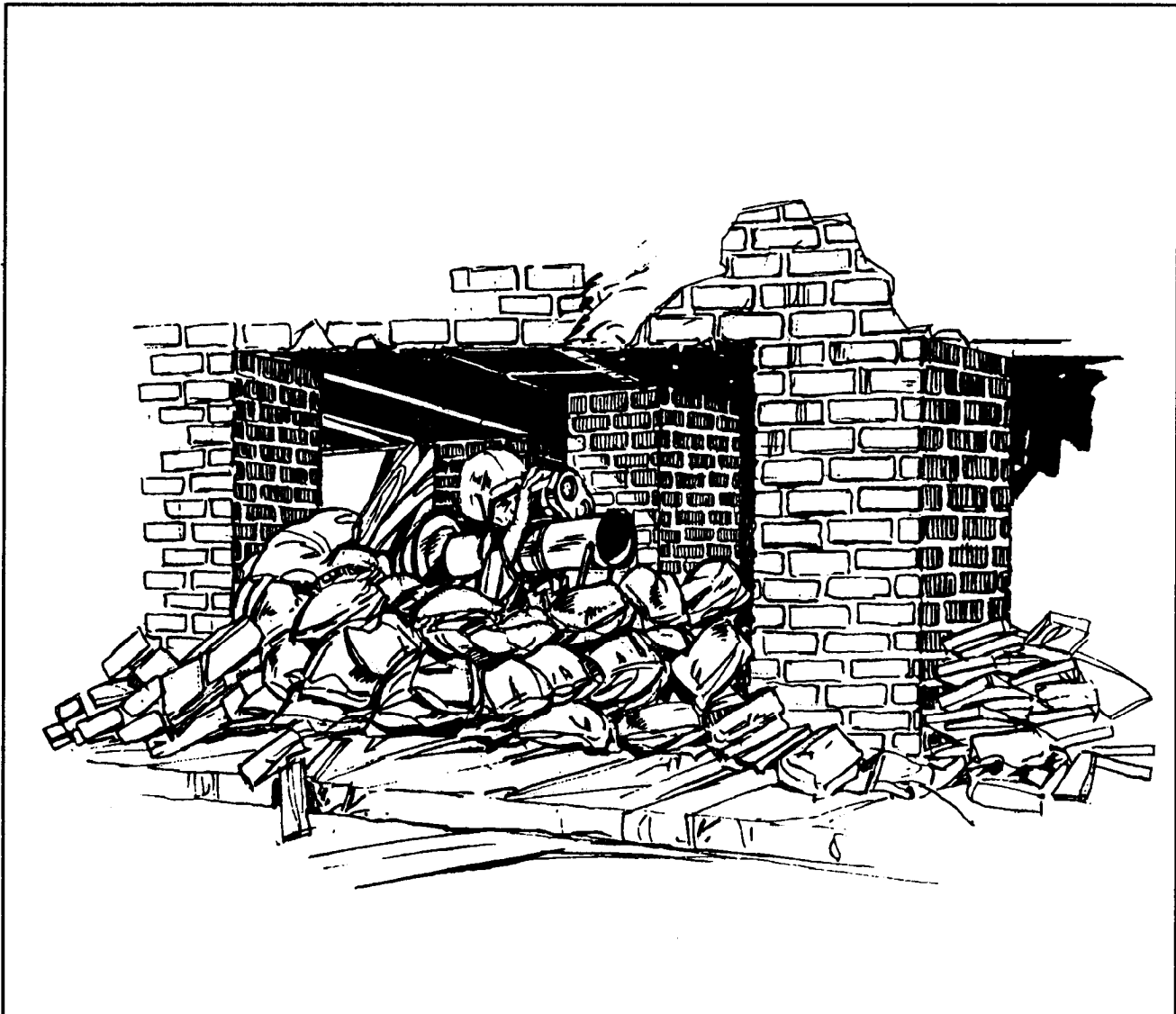
Figure 5-36. Prepared positions using a building for overhead cover.
