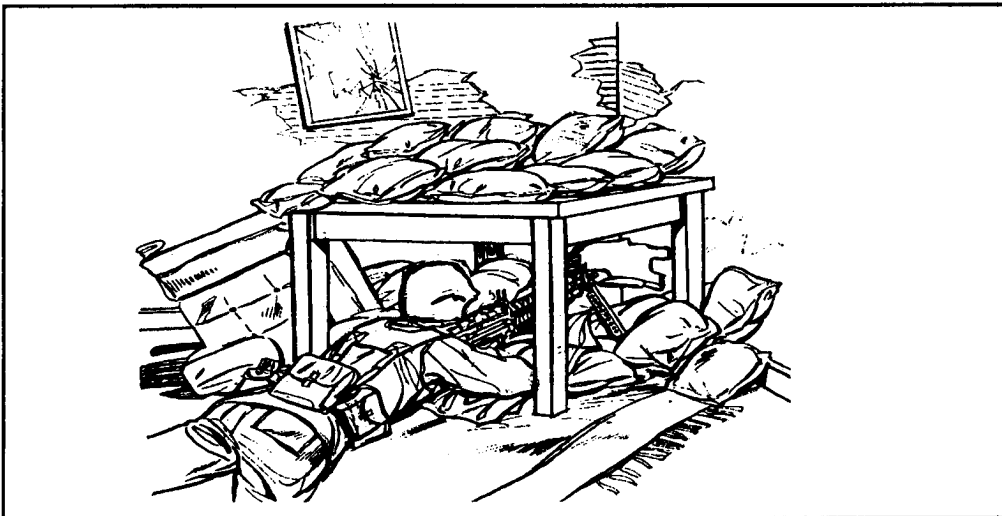
Figure 5-40. Corner machine gun bunker.
